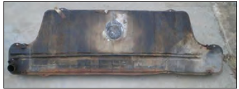
Rear repair - fuel tank You can see the damage on the right hand side - hopefully straightening will not create a leak!
