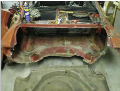
Tank removed Finally out, now I can clean up the damage and add the new section below - (thanks Guy)
